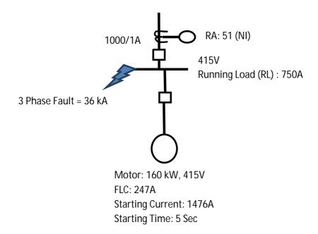
415V bus has maximum running load of 750A. The largest motor connected to this bus is 160 kW, DOL start motor.
