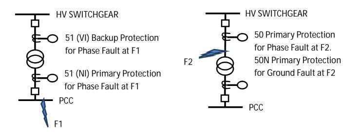
3.13Criteria for setting 50 (Instantaneous Overcurrent Protection) provided on transformer primary Case study: In one of the plant having 2 MVA transformer as shown below, the 50 relay setting was 9A. This unit operated for a 3 phase fault on one of the outgoing feeder as setting was incorrect.
