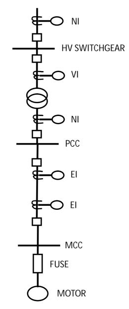
3.12Delta-Star (with grounded neutral)transformer with vector group Dyn11/Dyn1 shall be provided with 50, 51 and 50N protections on its primary side (Refer figure below):
