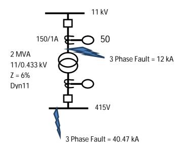
For a 3 phase fault on outgoing feeder, the current seen by relay =  $(40470 \times 433/11000) \times (1/150) = 10.62A$  which is above pick up setting of 9A. Hence relay operated instantaneously and tripped transformer HV breaker.
