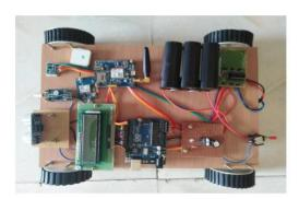
The hardware kit like a E-vehicle all the components are arranged as in the top view 4V battery three connected series with in to get 12V anything happens first shows the display through sim inserting send messages everything run over internet
