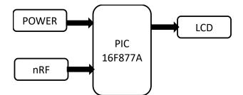
Fig:2 Block Diagram Of Receiver Unit
