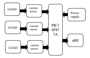
Fig:1Block diagram of Transmitter Unit
