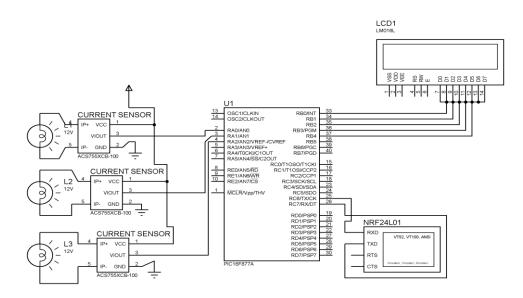
Fig:3 Circuit diagram of Transmitter Unit
