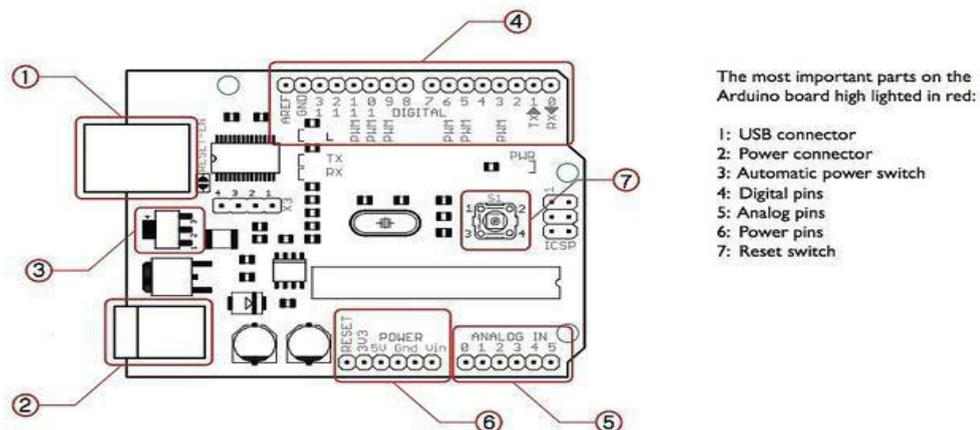
Figure 4.1. Arduino Pin Diagram
