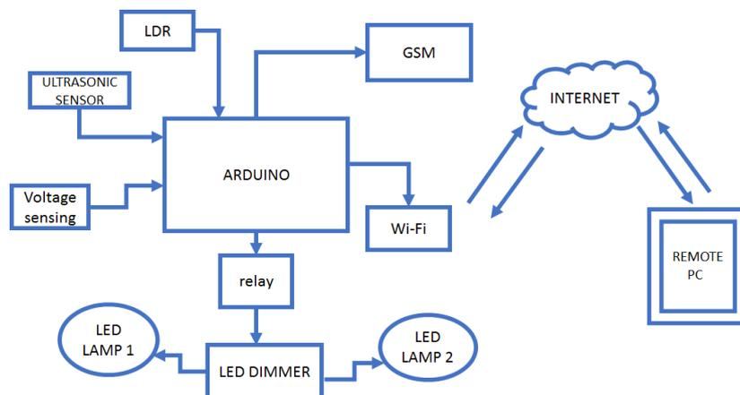
Figure 3.1 Project Block Diagram
