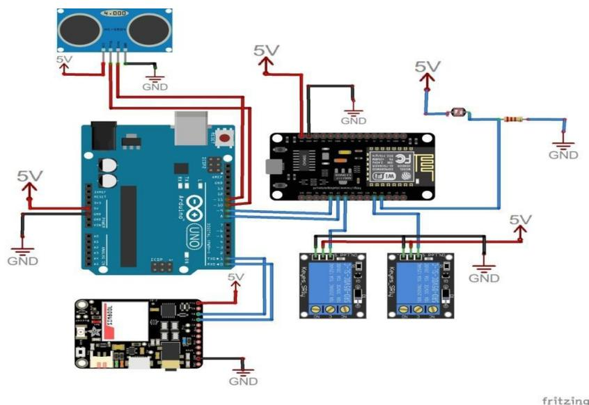
Figure 3.2 Project Circuit Diagram
