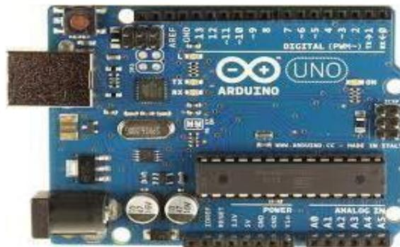
Fig-1 Arduino UNO Board
