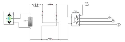
Fig.8 Z source inverter with PEMFC and Supercapacitor
