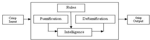
Fig.5 Basic Fuzzy logic controller
