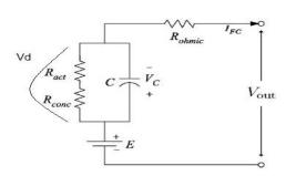
Fig.3 Equivalent Electrical circuit of PEMFC
