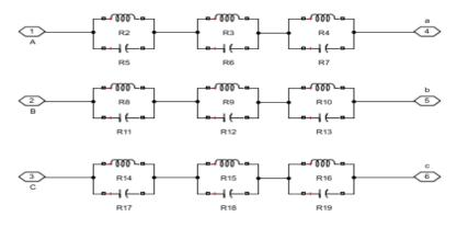
Fig.12 Passive filter
