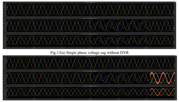
Fig.13(b) Single phase voltage sag compensation with DVR
