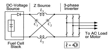
Fig.4 Three phase Z–Source Inverter
