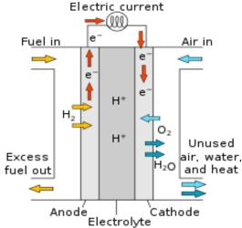
Fig.2. Basic operation of PEMFC
