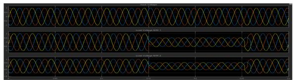
Fig.15(a) Three phase voltage sag without DVR
