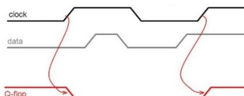
Fig. 3. Timing Diagram of Q flop
