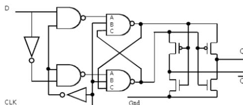
Fig. 1. Q flop with filter
