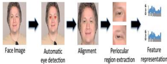
Fig 3: Frame work of periocular region extraction and representation
