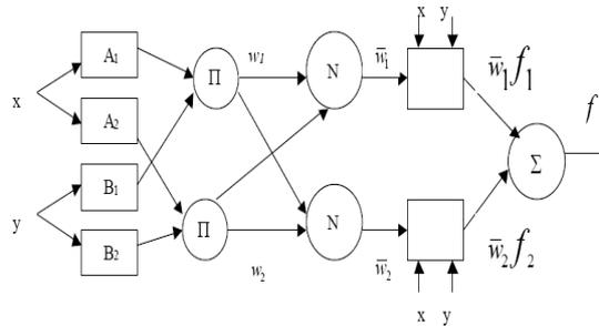
Figure 1: Structure of the ANFIS network.
