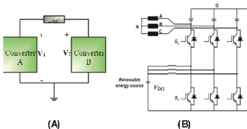
Figure 1 (a) Single-phase boost inverter block diagram and (b) three-phase boost inverter.
