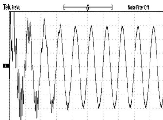
Figure 7 Inverter output voltage (10 V/Div, 20 ms/Div).
