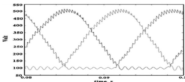
Figure: 3 Capacitors' voltage at  $M = 1.65$  and switching frequency of 3 kHz.
