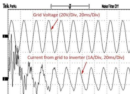
Figure 8 Channel 1: grid voltage, channel 2: current from grid to inverter.
