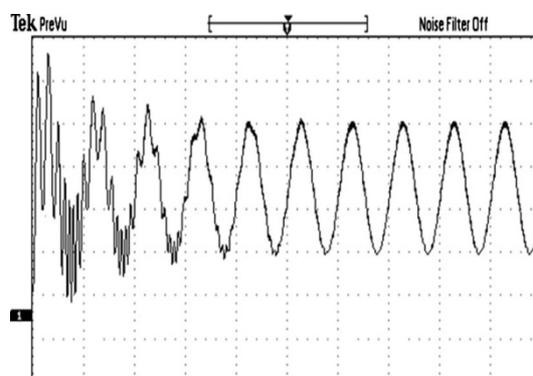
Figure 6 Capacitor voltage (20 V/Div, 20 ms/Div).
