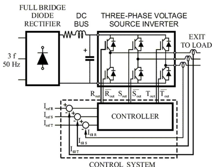
Figure: 2 three phase inverter single stage inverter
