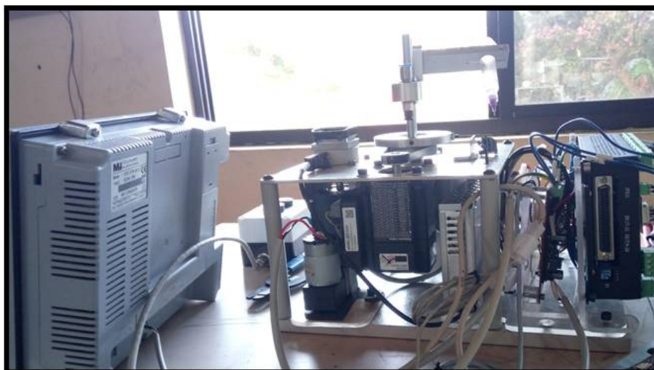
Fig. 3 Specially designed machine for adhesive dispensing on watch cases for fixing the dial cases
