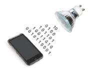
**Li-Fi** is a term often used to describe high-speed VLC in application scenarios where Wi-Fi might also be used. The term Li-Fi is similar to Wi-Fi with the exception that light rather than radio frequency wave is used for transmission.Li-Fi might be considered as complementary to Wi-Fi. If a user device is sited within a Li-Fi light bulb, it might be handed over from the Wi-Fi system to the Li-Fi system and there could be an enhancement in performance.
