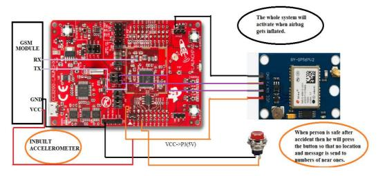
Fig. 2Circuit connection for the alert system
