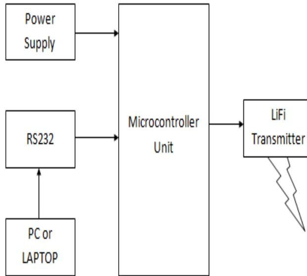
Fig.3 Block Diagram –Transmitter Unit
