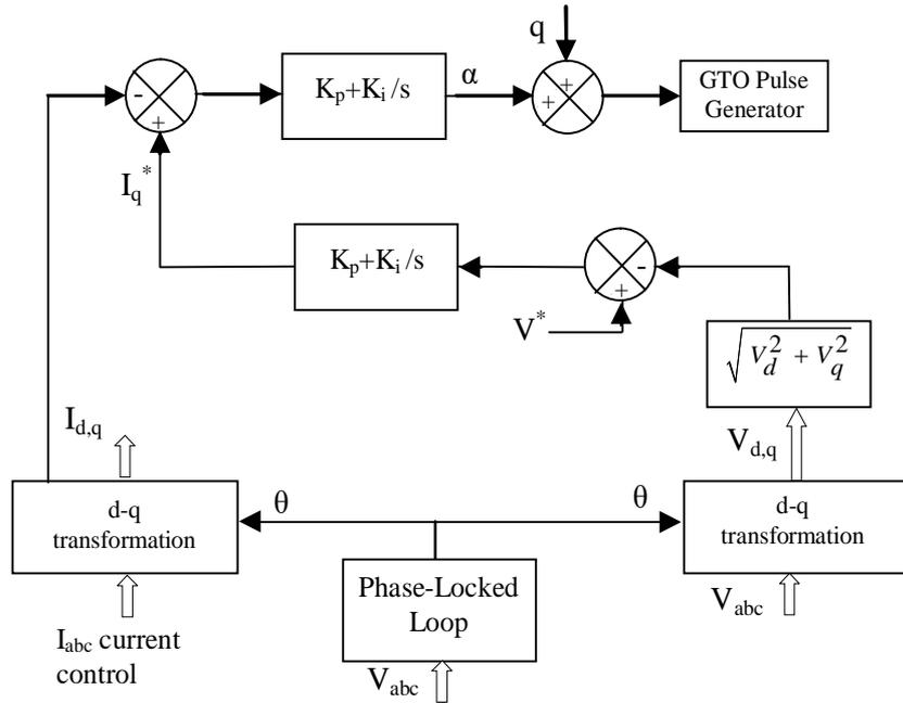
Fig. 5 STATCOM control schema
