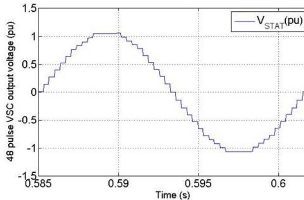
Fig. 4 48-pulse GTO-Converter output voltage
