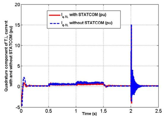
Fig. 17 Quadrature component of transmission line in pu
