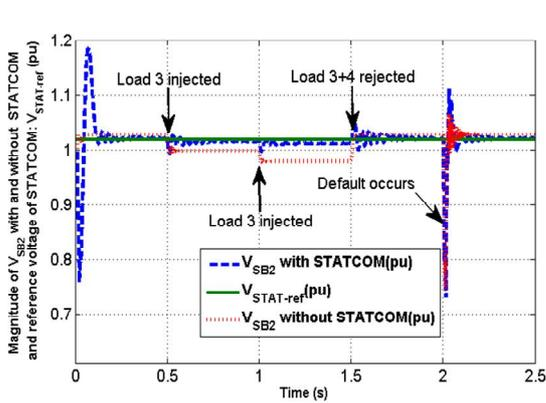
Fig. 8  $V_{ref}$  and  $V_{SB2}$  with and without STATCOM in pu
