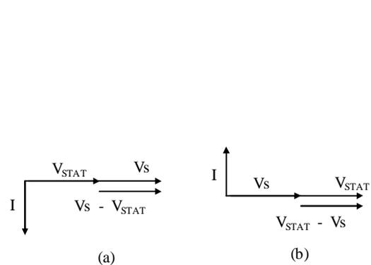
Fig. 2 STATCOM main operation: (a) inductive operation, (b) capacitive operation
