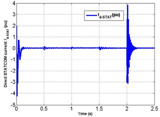
Fig. 11 Direct component of STATCOM current in pu
