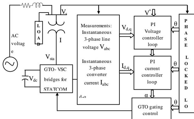
Fig. 1 GTO-VSC based STATCOM architecture
