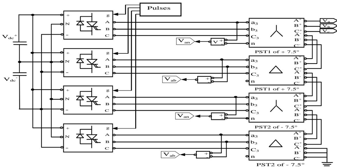
Fig. 3 Circuit layout of the proposed 48-pulse STATCOM configuration
