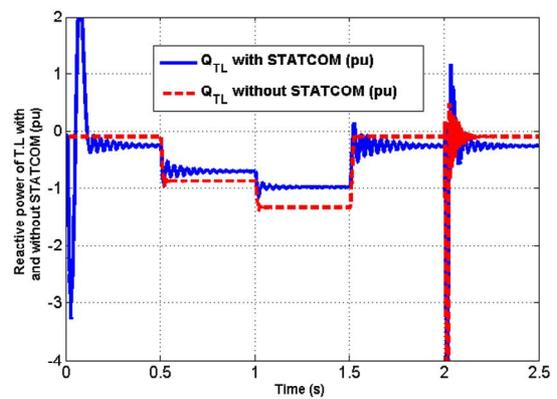
Fig. 15 Reactive power of transmission line in pu
