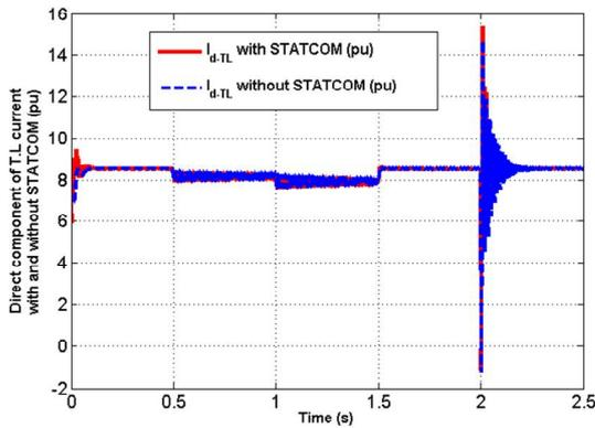
Fig. 16 Direct component of transmission line current in pu
