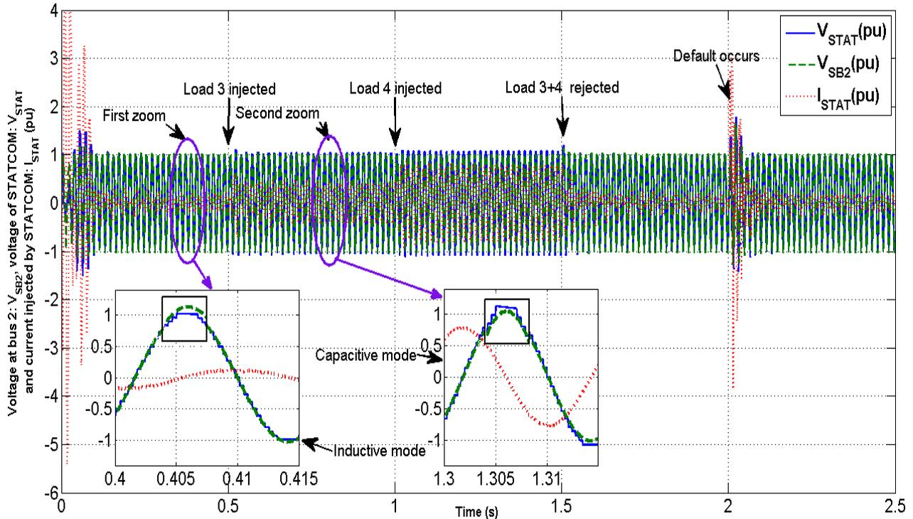
Fig. 7 Voltage of bus 2, STATCOM voltage and STATCOM in pu
