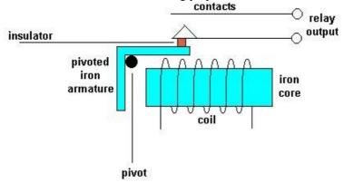
Fig7. Relay Circuit
