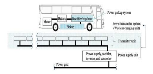
Poor coupling can result in poor transmission performance and low efficiency. Due to the large air gap between the primary and secondary windings, contactless transformers have large leakage inductances, small mutual inductance and low efficiency. Compared to direct contact charging, inductive charging efficiency is lower and resistive heating is.
