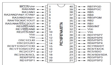
Fig4. Pin Diagram of PIC 16F877A
