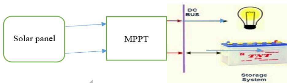
Figure 1.4 Micro grid Architecture
