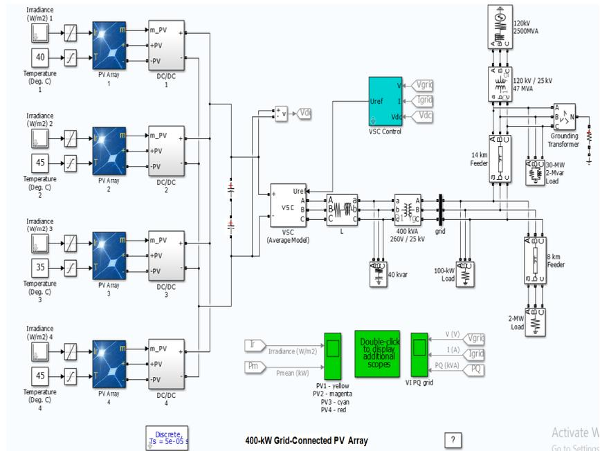
Figure 1.5 Matlab/ Simulink model of 400 kW PV array Micro grid.
