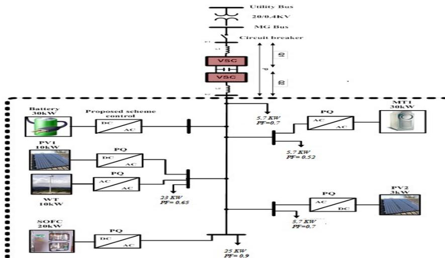
Figure 1.1 single line diagram of the micro grid system
