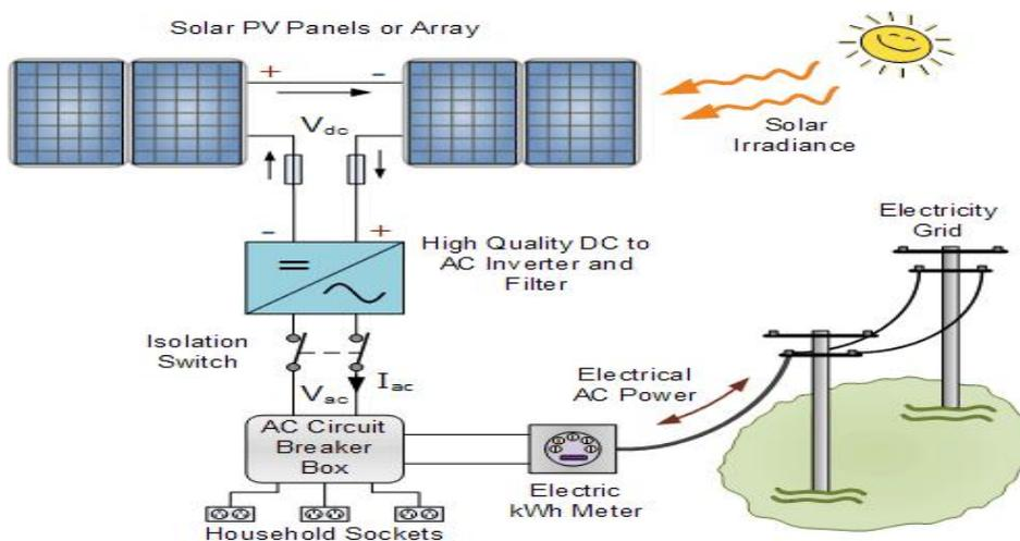
Figure 1.2: Micro Grid connected PV system (Source MNRE 2011)
