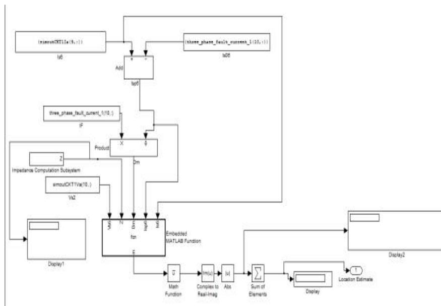
Figure 3: Fault location subsystem.
