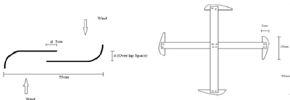
Fig. 2. Savonius and Darrieus Turbine
