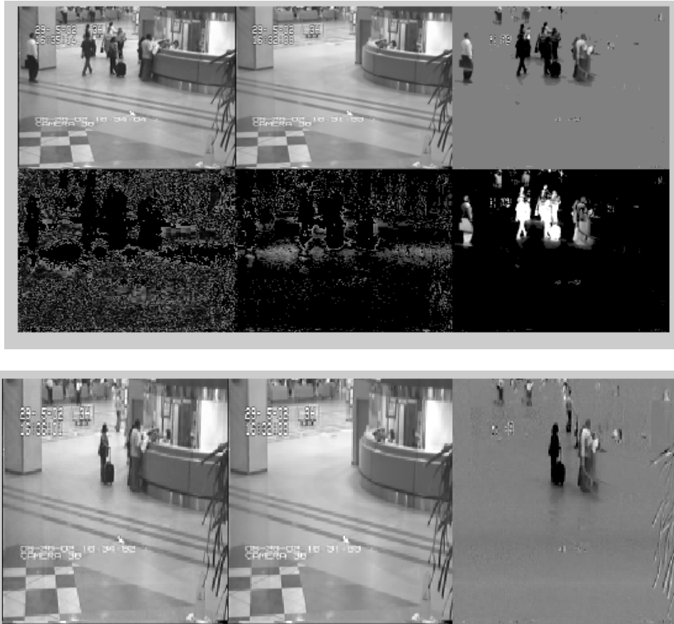
Fig. 4. Performance of OMoGMF on video sequences with missing entries. From upper to lower: Original video frames, 15% subsampling frames, extracted backgrounds.
