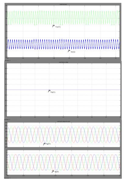
Fig.6. Response of the system in the absence of wind source while PV source continues to operate at MPPT.
