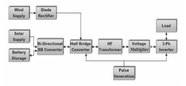
Fig. 1 Grid connected hybrid system with voltage multiplier for three phase applications.
