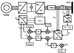
Fig. 1 Control of grid side converter for voltage regulation
