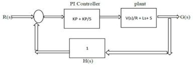
Fig. 2 Block diagram of PI controller
