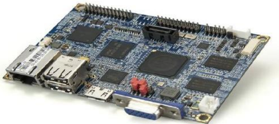
Fig. 1: VIA VAB-800 10 cm x 7.2 cm Pico-ITX Embedded ARM Board
