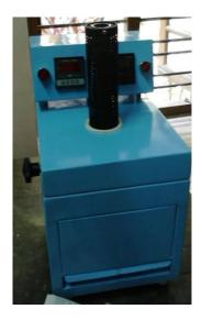
The unit is constructed of a double jacketed chamber with ceramic insulator filled in between the two chambers. The door is provided at the top portion and the micro switch to count the number of opening and closing of door is fixed at the hinges. A front sliding pan is provided at the bottom region from the ash is collected. The electronic circuitry and controls are provided on the top panel. The funnel for smoke emission is provided along with the top door.
