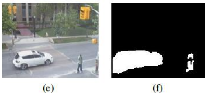
Fig 1: Different cases of ANC. Figs (a), (b) show that ANC detects foreground partially and figs (c),(d) show that ANC cannot remove repetitive motions well. Also figs. (e), (f) show that ANC detects following of moving objects wrongly.
