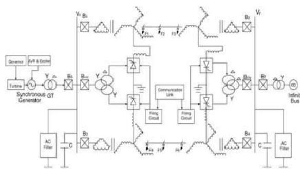
Fig 1. Basic circuit diagram of simultaneous Ac-dc transmission
