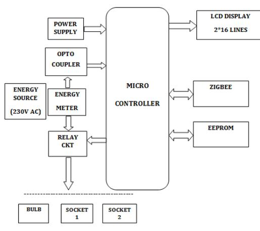
Fig 1: Monitoring section
