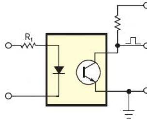
Fig 3: Optocoupler structure
