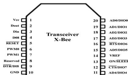
Fig 4: ZIGBEE pin diagram
