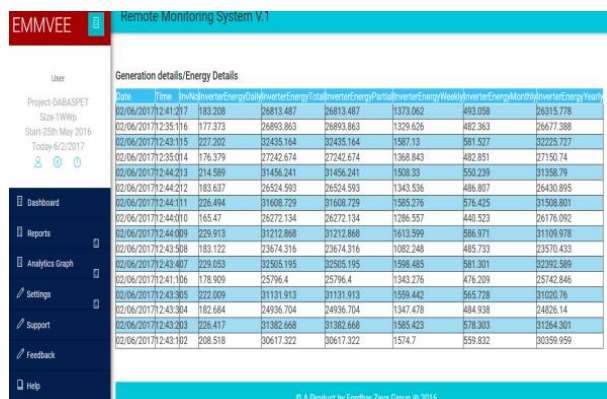
Figure 5 Individual inverters generation details
