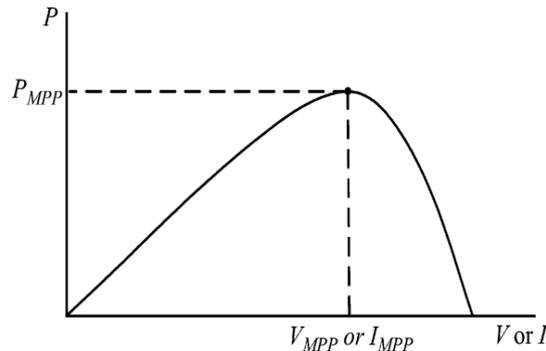
Fig.1 Characteristics PV array power curve
