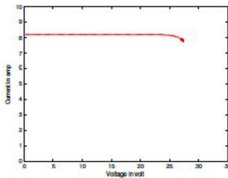
Fig 6. V-I Characteristics of P & O Algorithm
