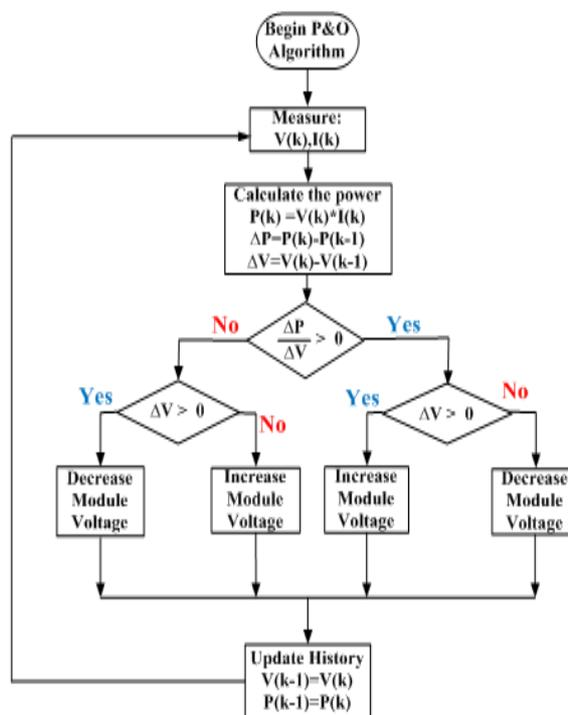
Fig 3. Flowchart of P & O Algorithm
