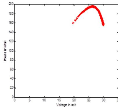
Fig 11. P- V Characteristics of Adaptive P&O
