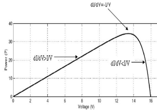
Fig. 4. P/V characteristics of Incremental conductance
