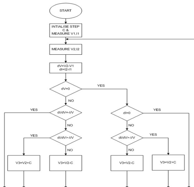
Fig 5. Flowchart of Incremental conductance algorithm
