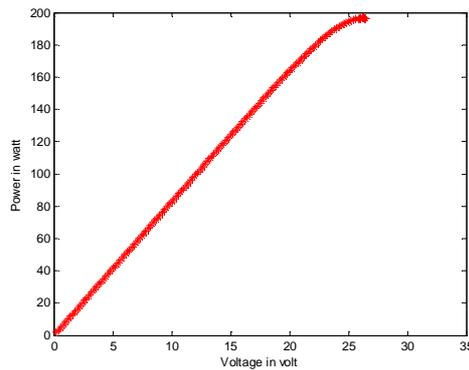
Fig 9. P-V Characteristics of Incremental Conductance
