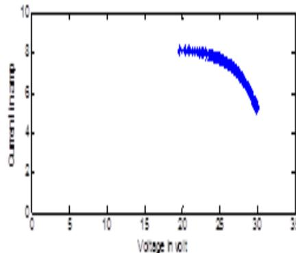
Fig 10. V-I Characteristics of Adaptive P&O
