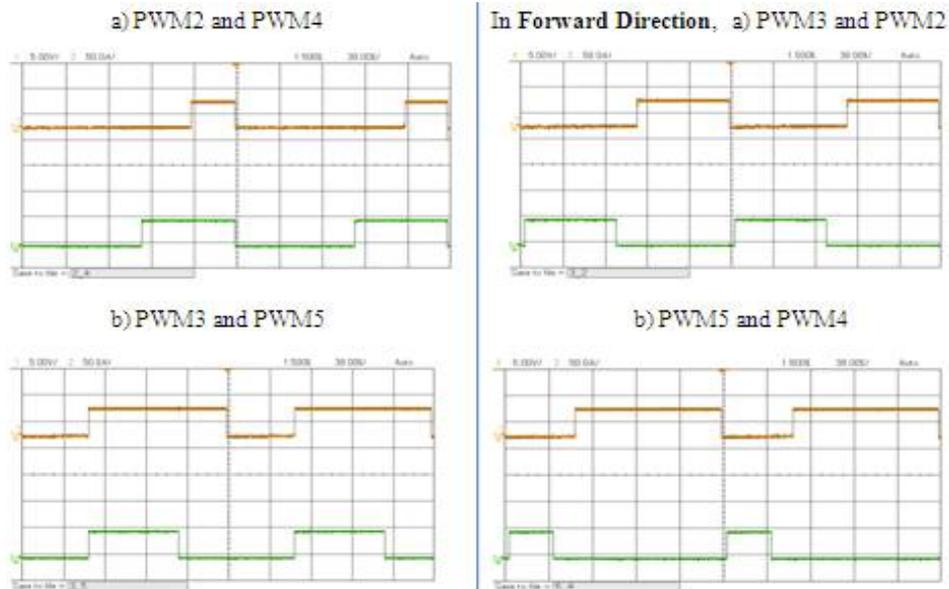
Fig. 6.5: Comparison of PWM2 and PWM3 with PWM4 and PWM5 at ADC=27
