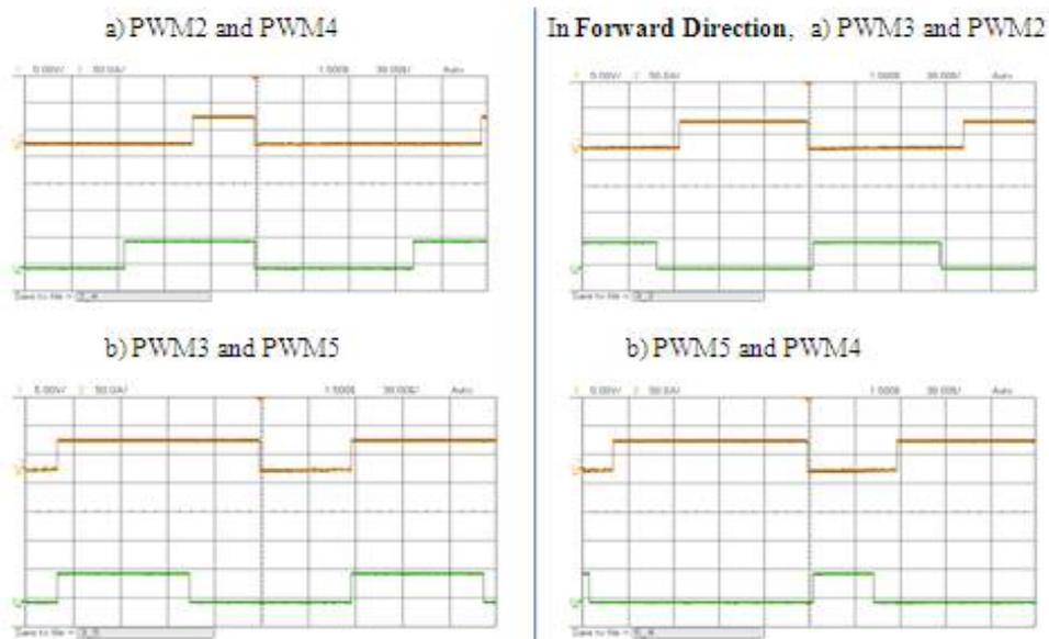
Fig. 6.6: Comparison of PWM2 and PWM3 with PWM4 and PWM5 at ADC=504
