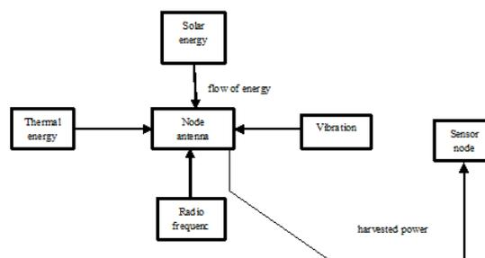
Fig.1 Different Types of Sources for Energy Harvesting By Sensor Device.
