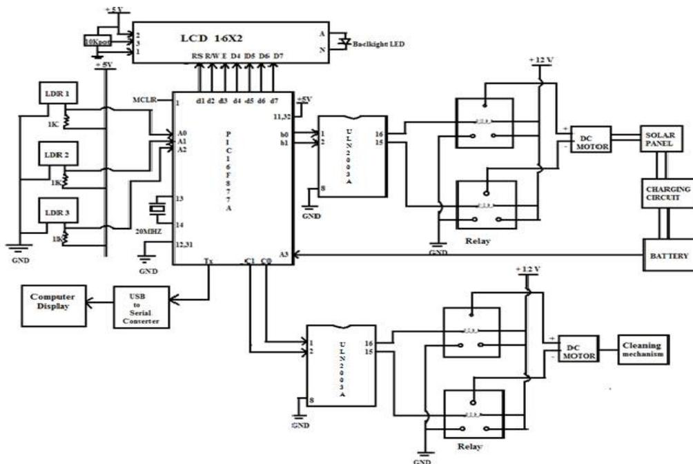
Fig:5: Functional connection diagram
