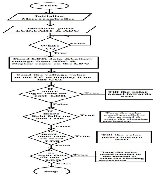
Fig: 4 flow chart of the auto cleaning system
