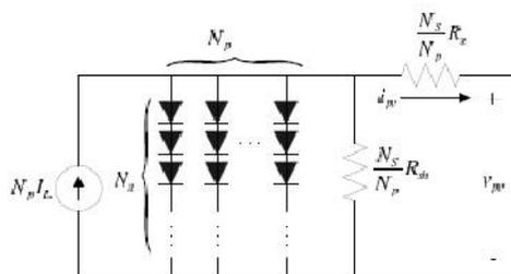
Fig. 3. Equivalent circuit diagram of PV array
