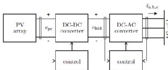
Fig. 1. Block diagram of the PV system.
