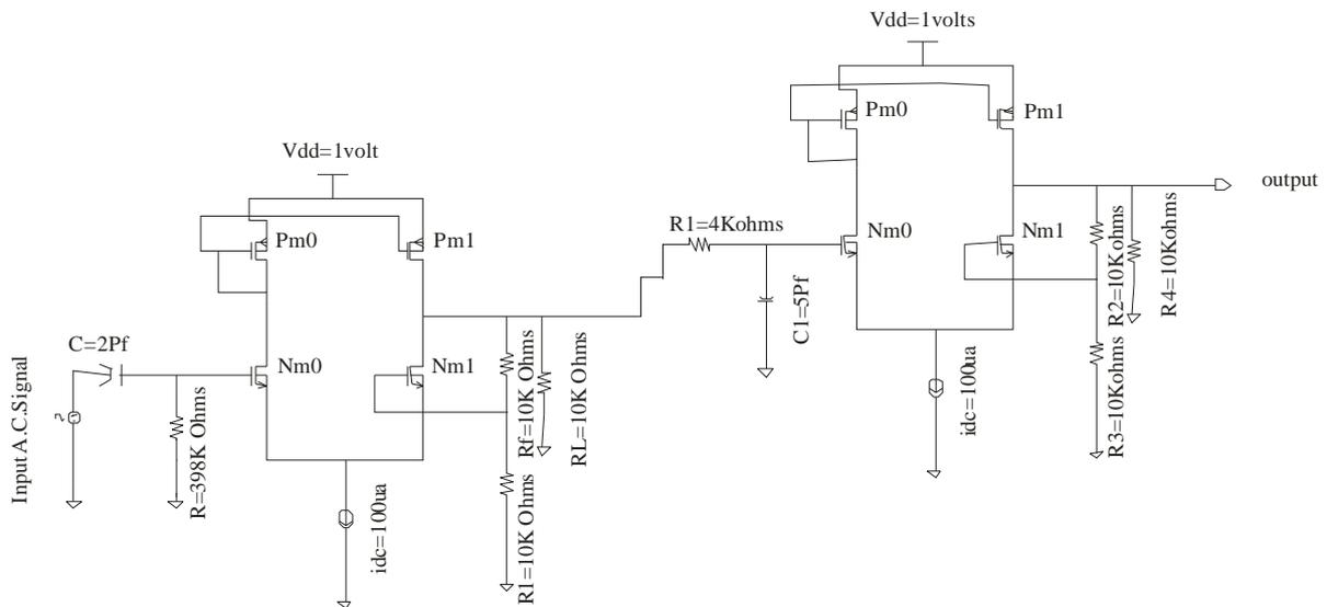
Figure 2. Conventional Active Band Pass Filter.
