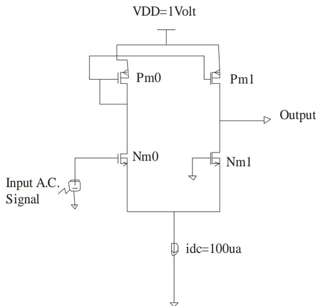
Figure 1. Single Stage CMOS Operational Amplifier.
