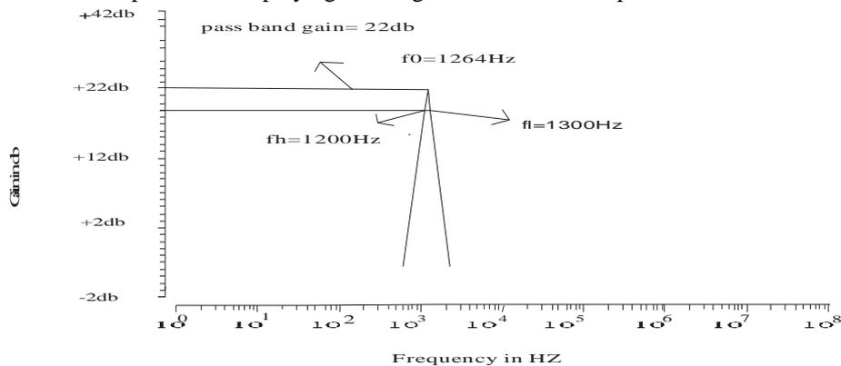
Figure 7. Frequency Response of Proposed Active Band Pass Filter.
