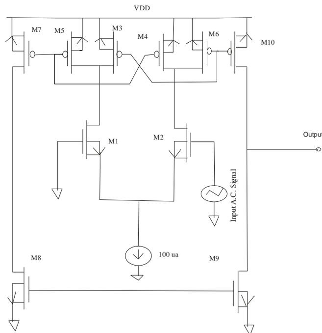
Figure 3. Two Stage OPAMP with Positive Feedback.
