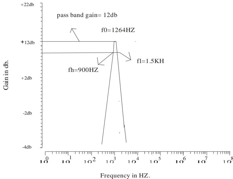
Figure 6. Frequency Response of Active Band Pass filter employing Positive Feedback.
