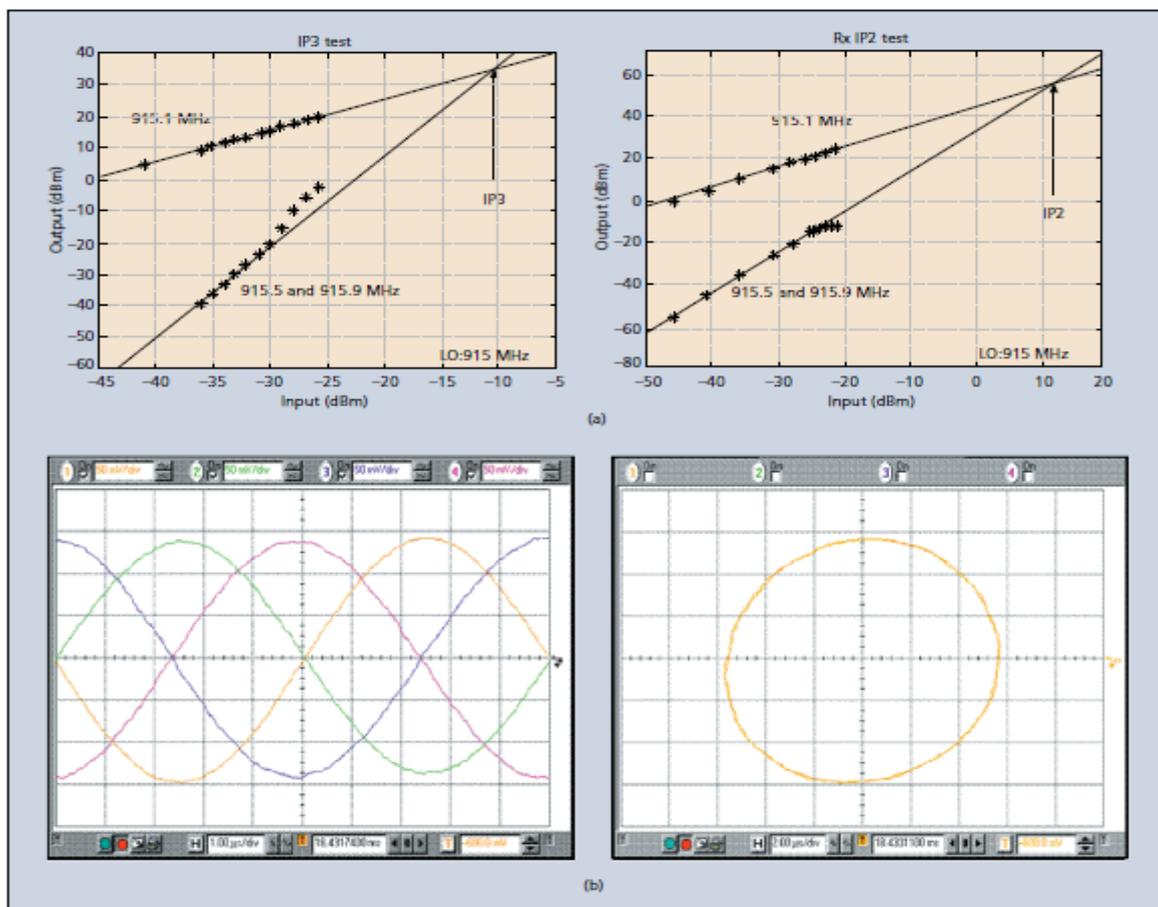
Figure 3. Measured receiver characteristics and a) IIP3 and IIP2 values; b) baseband output I/Q waveform and I vs. Q diagram.
