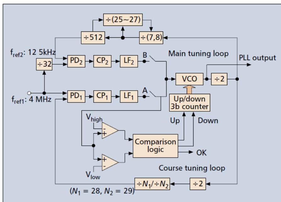
Figure 2. The PLL block diagram.
