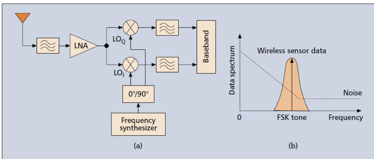
■ **Figure 1.** a) A direction-conversion receiver architectural block diagram; b) the downconverted FSK signal spectrum, indicating large tone frequency reducing flicker noise impact.
