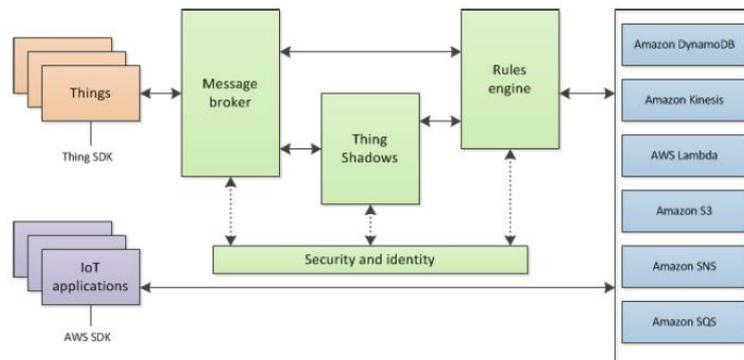
Figure 6: Simplified view of AWS IoT
