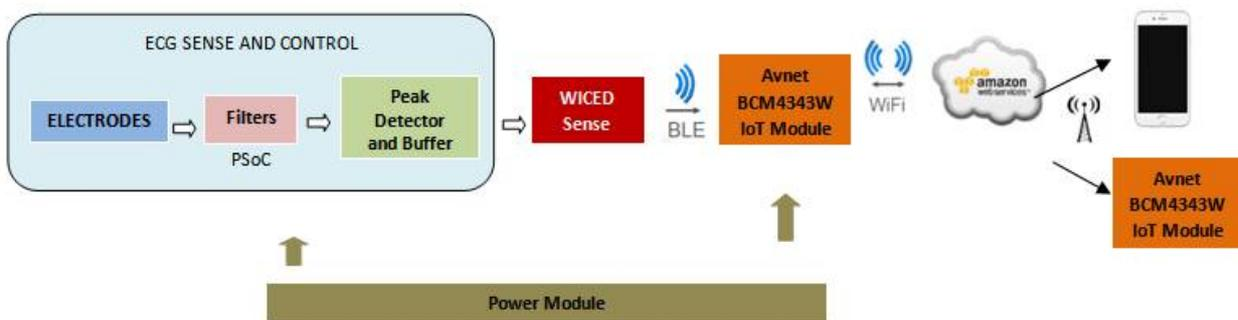
Figure 3: Block diagram IOT based ECG monitoring system
