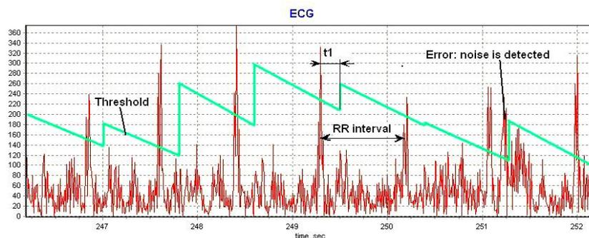
Figure 7: ECG thresholding and noise detection
