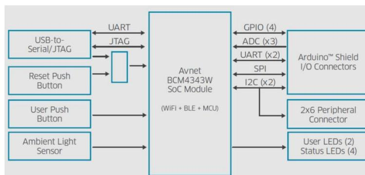
Figure 4: BCM4343W IOT starter kit block diagram
