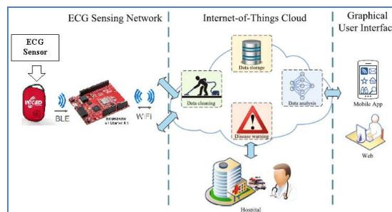
Fig. 1 Architecture of the IoT-based ECG monitoring system.
