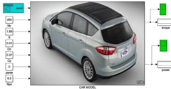
Fig 3 :simulink model of a solar vehicle with acceleration forces
