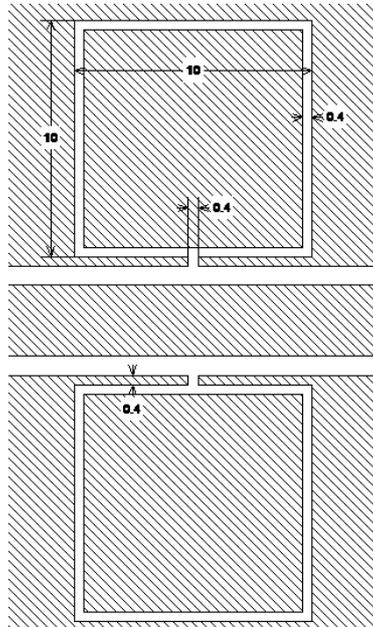
Fig. 1. Layout of a modified dumbbell-shaped DGS with mm as the unit.
