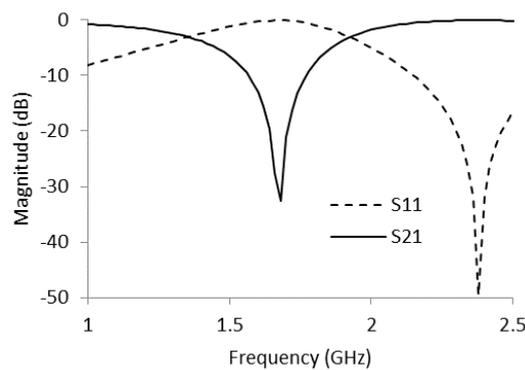
Fig. 4. Simulation results of the CM-DGS.
