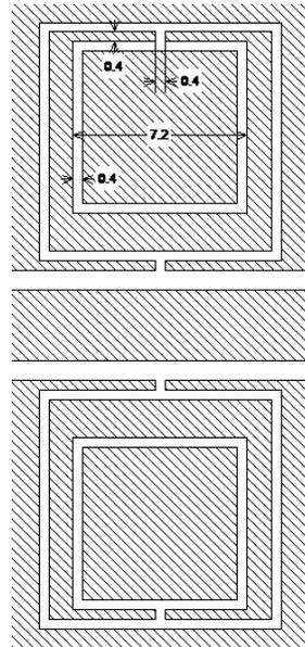
Fig. 3. Layout of a CM-DGS with mm as the unit.
