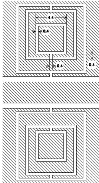
Fig. 5. Layout of the new CM-DGS with three square loops.
