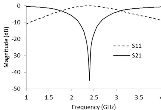
Fig.2. Simulation results of the modified dumbbell-shaped DGS
