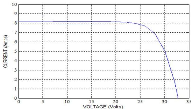
Fig 1.16 V-I curve of PV module
