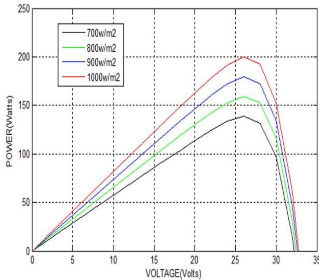
Fig 1.19 Effect of Variation of Irradiation on P-V Characteristics
