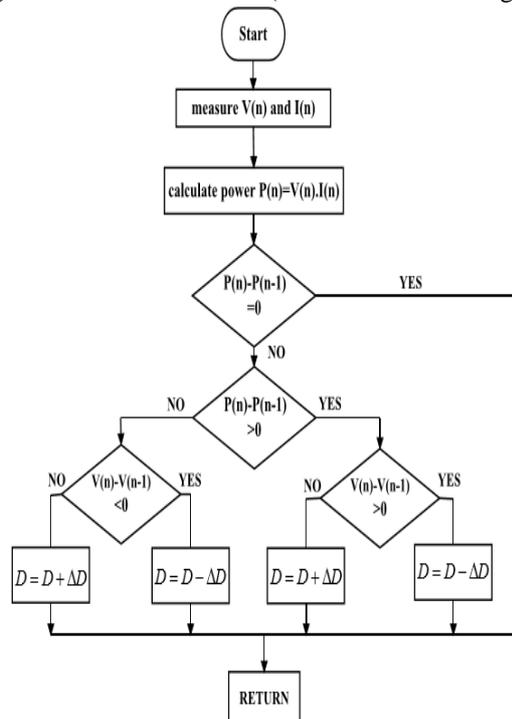
Fig 1.9 Flowchart of Perturb & Observe MPPT algorithm
