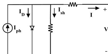
Fig 1.4 Equivalent circuit of Single diode model of a solar cell
