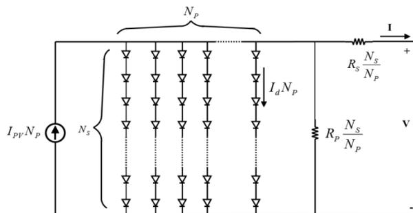
Fig 1.5 Representation of PV module
