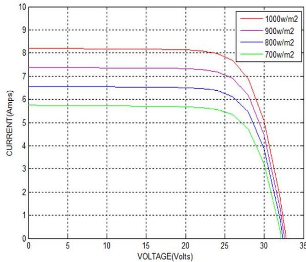
Fig 1.18 Effect of Variation of Irradiation on I-V Characteristics
