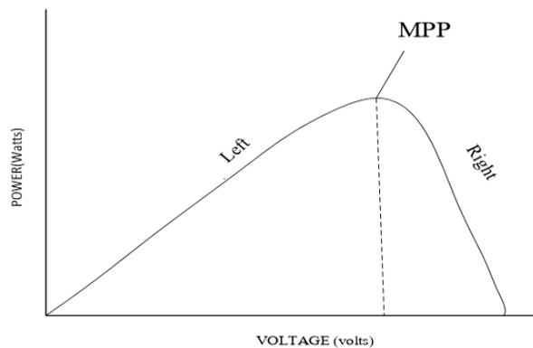
Fig. 1.8 P-V characteristics (basic idea of P&O algorithm)
