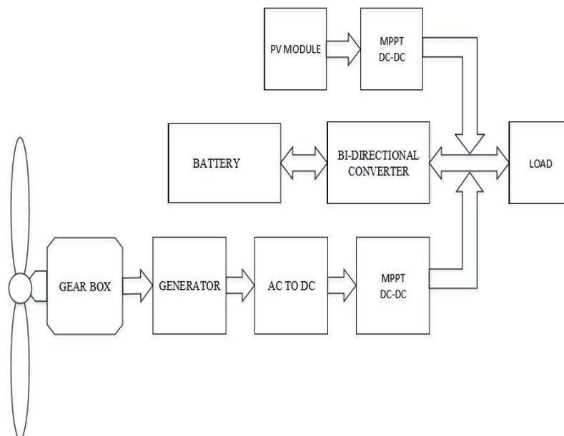
Fig 1.2 Block diagram of hybrid system
