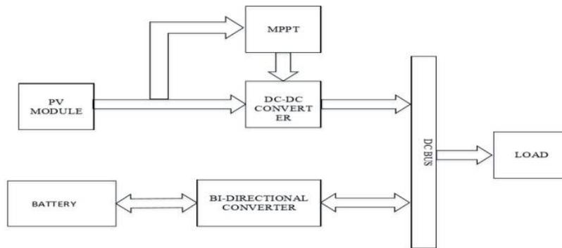
Fig 1.3 Overall Block Diagram of PV Energy System
