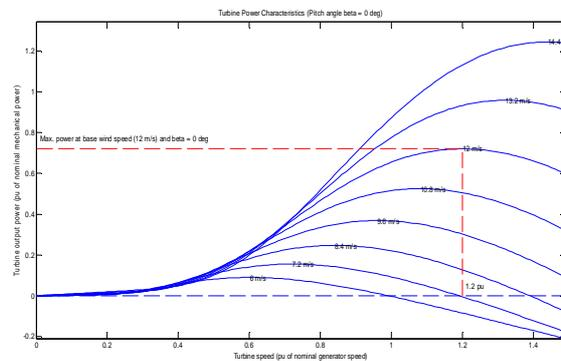
Fig 1.22 Turbine Power Characteristics (pitch angle  $\beta=0^\circ$ )
