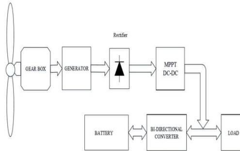
Fig 1.10 Overall Block Diagram of Wind Energy System
