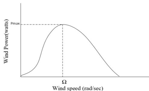
Fig 1.11 Powers vs. Speed Characteristics of Wind Turbine
