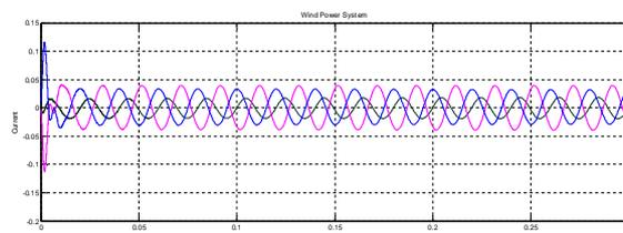
Fig 1.24 Three Phase Line Output Current of Wind System
