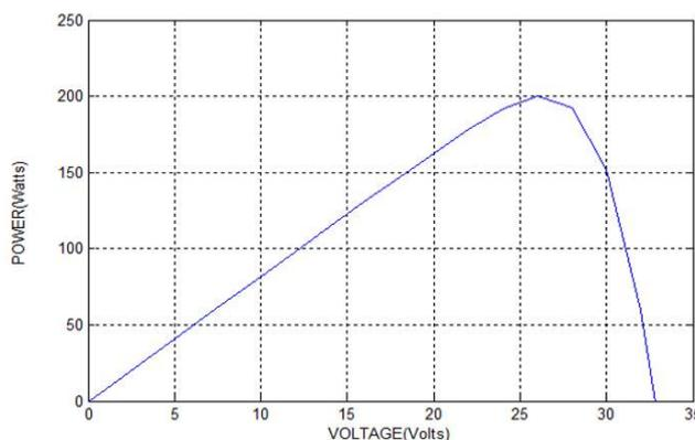
Fig 1.17 P-V curve of PV module
