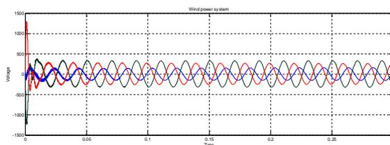
Fig 1.23 Three Phase Line Output Voltage of Wind System
