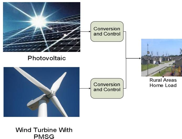
Figure 1.12 - Block diagram of the developed hybrid power system
