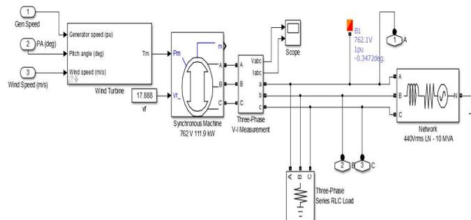
Figure 1.14 – Implementation of the Wind Turbine PMSG Model
