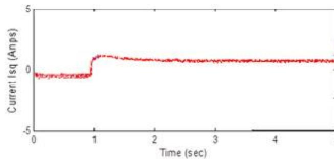
Figure5b: Current response of the PMSM with the proposed controller under no load.
