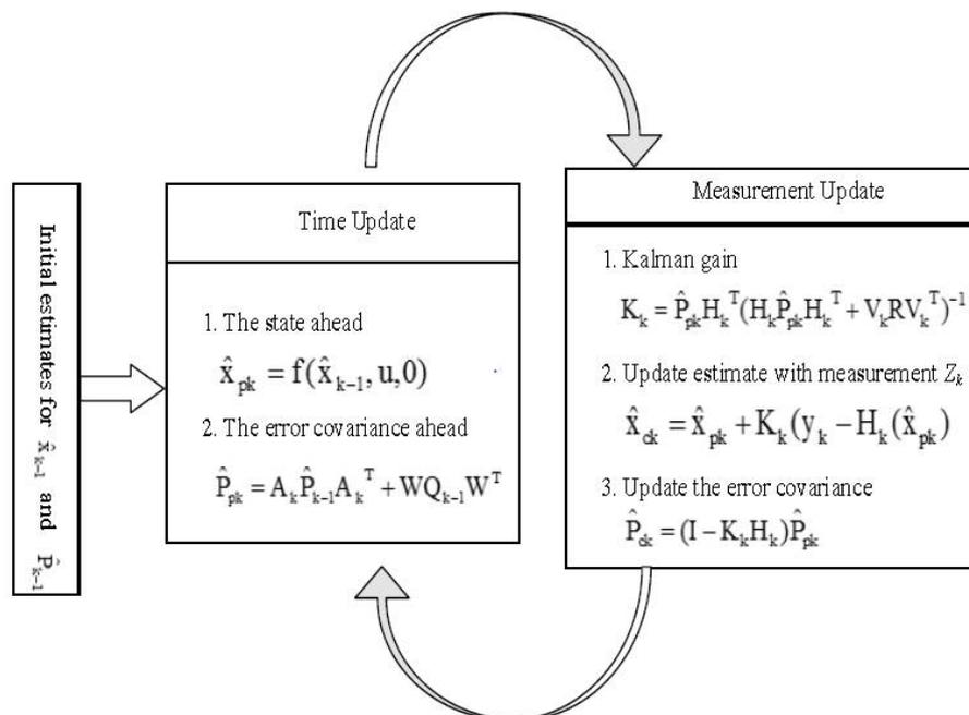
**Figure 1: The Kalman filter algorithm.**
