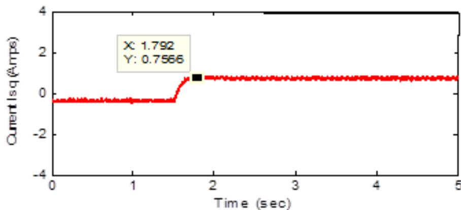
Figure7b: Current response of the PMSM with the proposed controller under increasing load.
