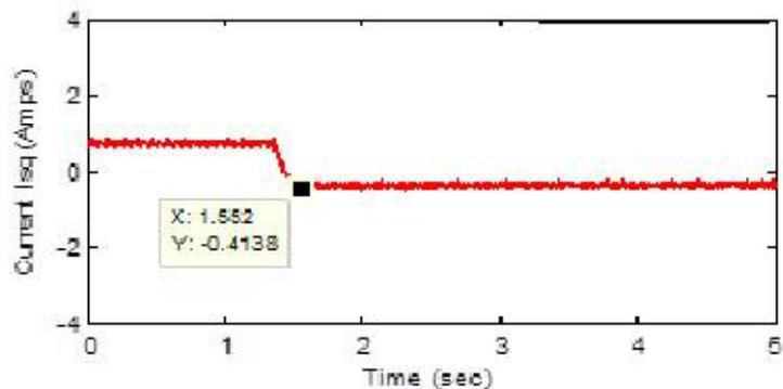
Figure 9b: Current response of the PMSM with the proposed controller under decreasing load.
