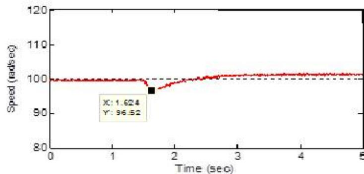
Figure6b:Speed response of the PMSM with the proposed controller under increasing load.
