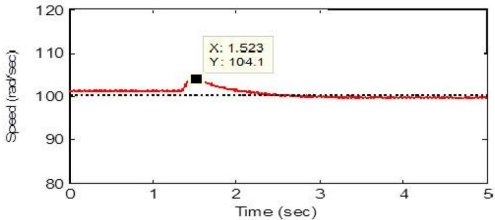
Figure 8b: Speed response of the PMSM with the proposed controller under decreasing load.
