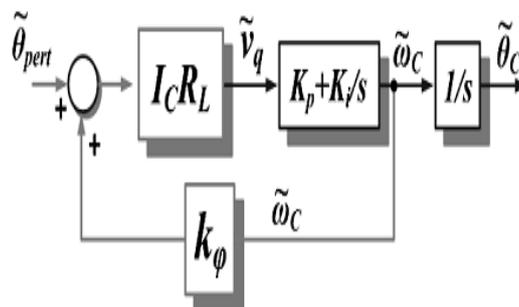
Fig. 5. Linearized small-signal PLL model under islanded condition.
