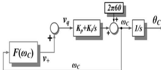
Fig. 4. SRF PLL model under the islanded condition.
