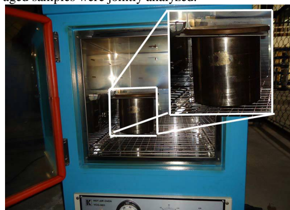
(b) Test set up for thermal faults [32]
