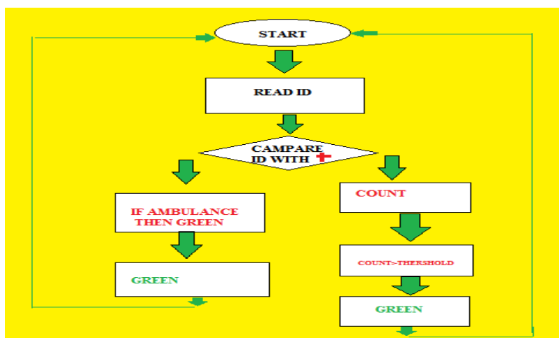
Fig.3: Flow diagram for Congestion control
