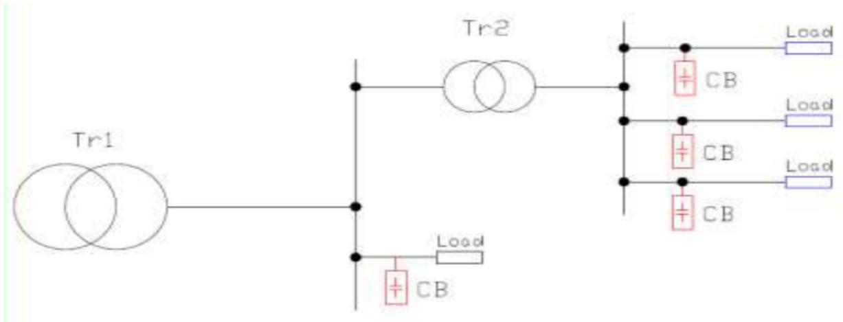
Fig 1. Illustration of fixed power factor correction
