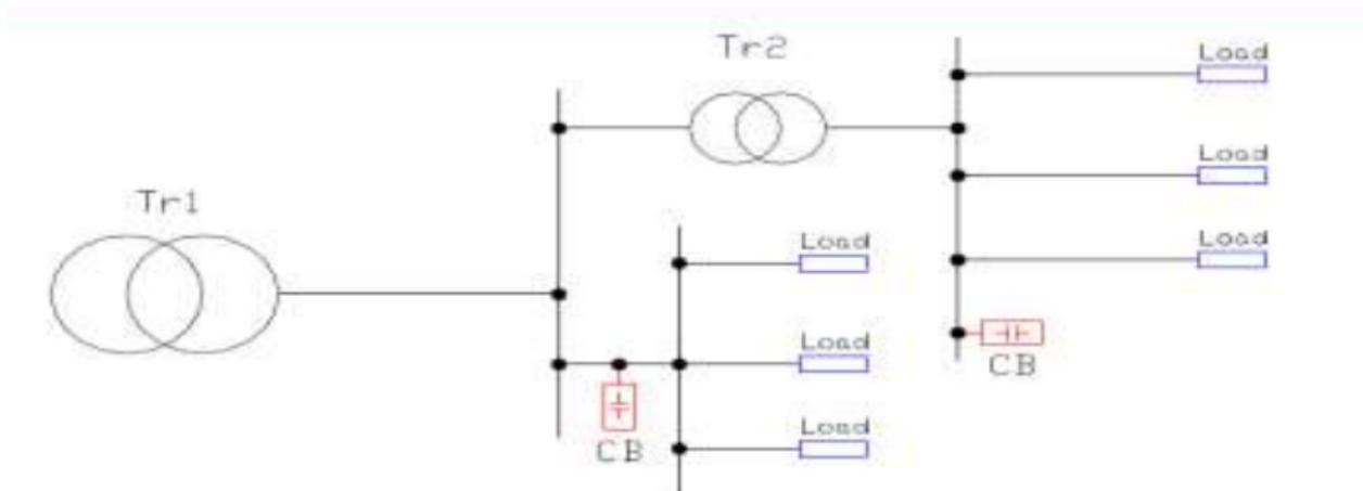
Fig 2. Illustration of group power factor correction
