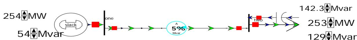
Fig 5. power flow diagram with 142.3MVAR connected in parallel
