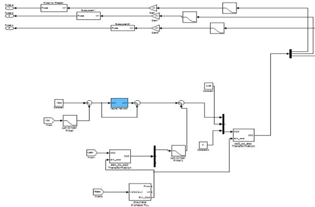
Fig. 5- MATLAB/SIMULINK Diagram of the reference current extraction using Neural Network based SRF theory.
