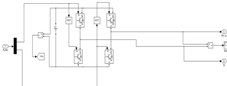
Fig.- Single phase three level H-Bridge Cascaded Multi Level Inverter
