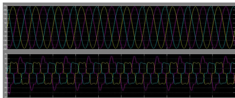
Fig.9- Load voltage and current without compensation (NN)
