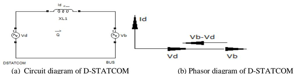
Fig.3-Capacitive mode of D-STATCOM
