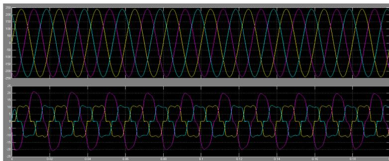
Fig.10- Load voltage and current with compensation (NN)
