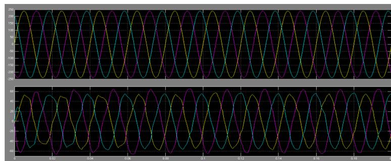
Fig.8- source voltage and current with compensation(neural network)
