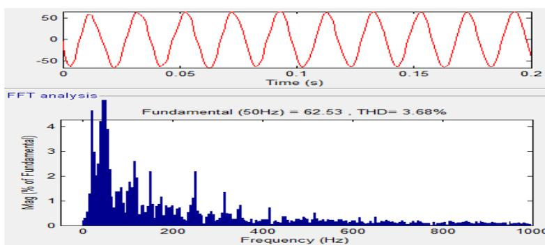
Fig.14- Supply current phase-B Waveform & %THD with compensation
