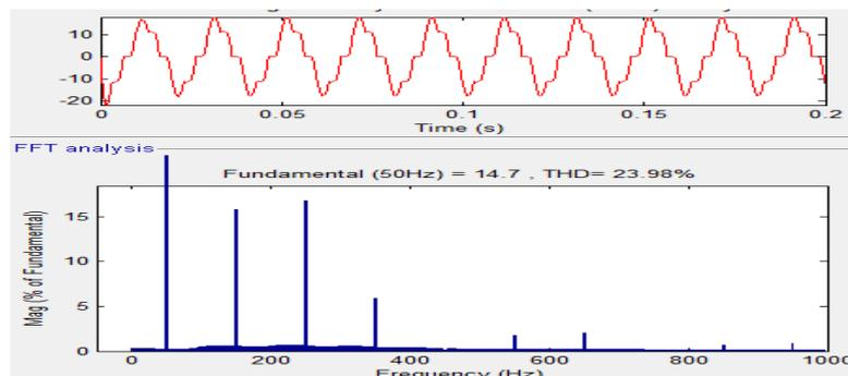
Fig.12- Supply Current phase-B Waveform & %THD without compensation
