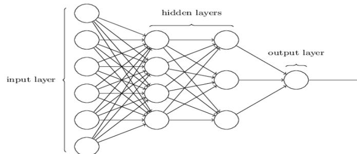
Fig.6-Basic Neural Network diagram
