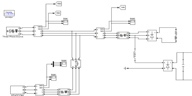
Fig.4-Proposed Neural Network based MLI-DSTATCOM of 3-phase 4 wire system
