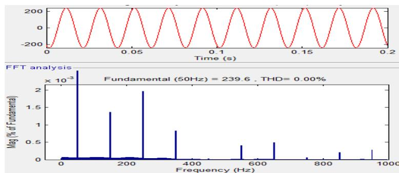
Fig.11- Supply voltage phase-B Waveform & %THD without compensation
