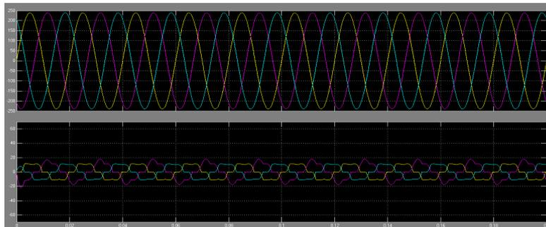
Fig.7- source voltage and current without compensation (NN)
