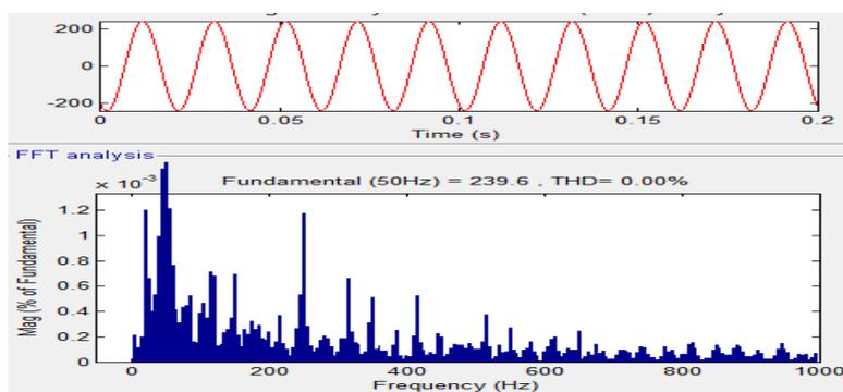
Fig.13- Supply voltage of phase-B Waveform & %THD with NN controller
