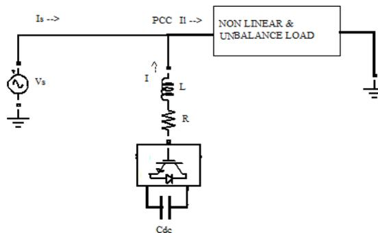
Fig.1- Single line diagram of DSTATCOM
