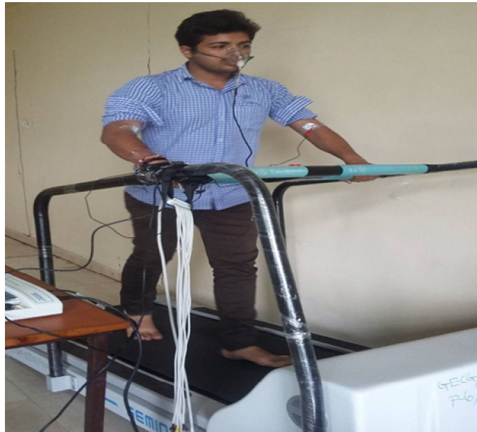
Fig. 1 Cardiopulmonary exercise testing using treadmill machine. Continues ECG and respiration rate monitoring using thermistor sensor.
