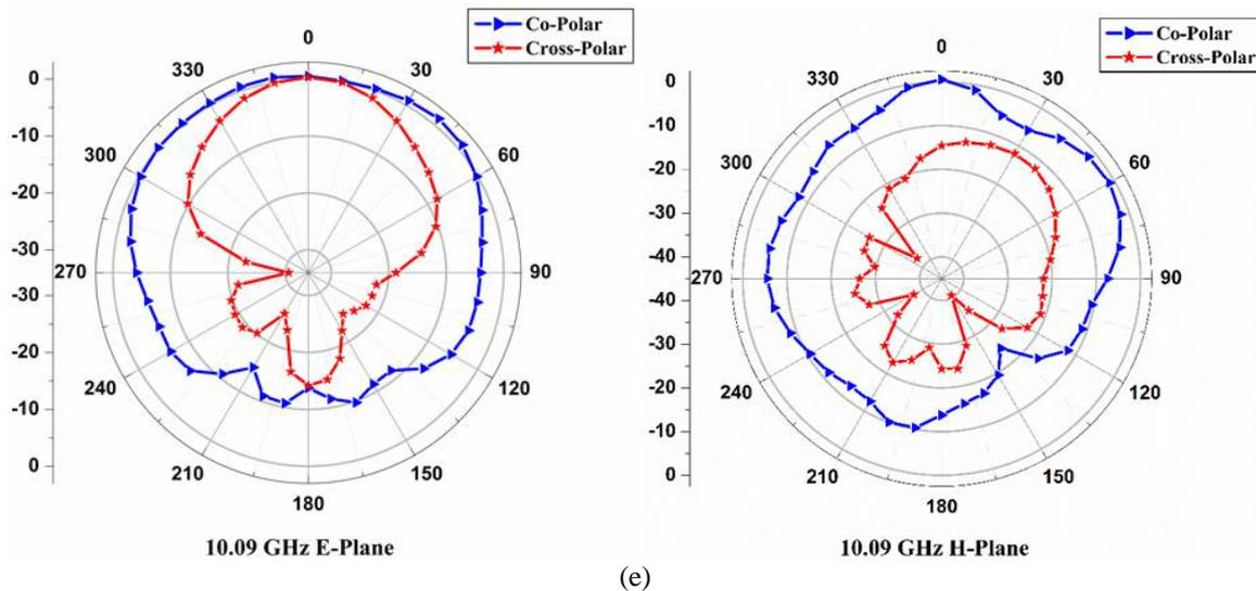
Fig. 4 Typical co-polarization and cross-polarization in E-plane and H-plane radiation patterns of the proposed antenna measured at (a) 2.33 GHz, (b) 3.44 GHz, (c) 8.13GHz, (d) 8.67 GHz and (e) 10.09 GHz
