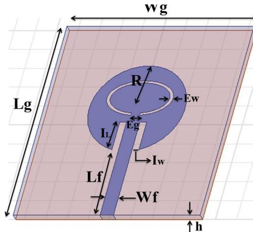
Fig. 1 Geometry of the proposed inset-fed circular microstrip antenna
