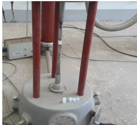
Fig.(4): Unsaturated Polyester insulator with Nano fillers during test
