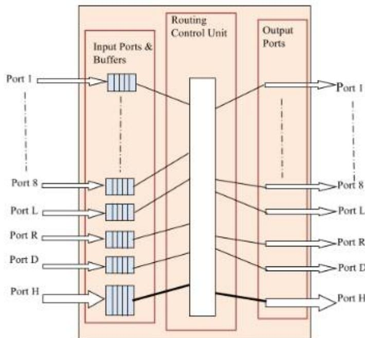
Fig. 7 Router internal architecture
