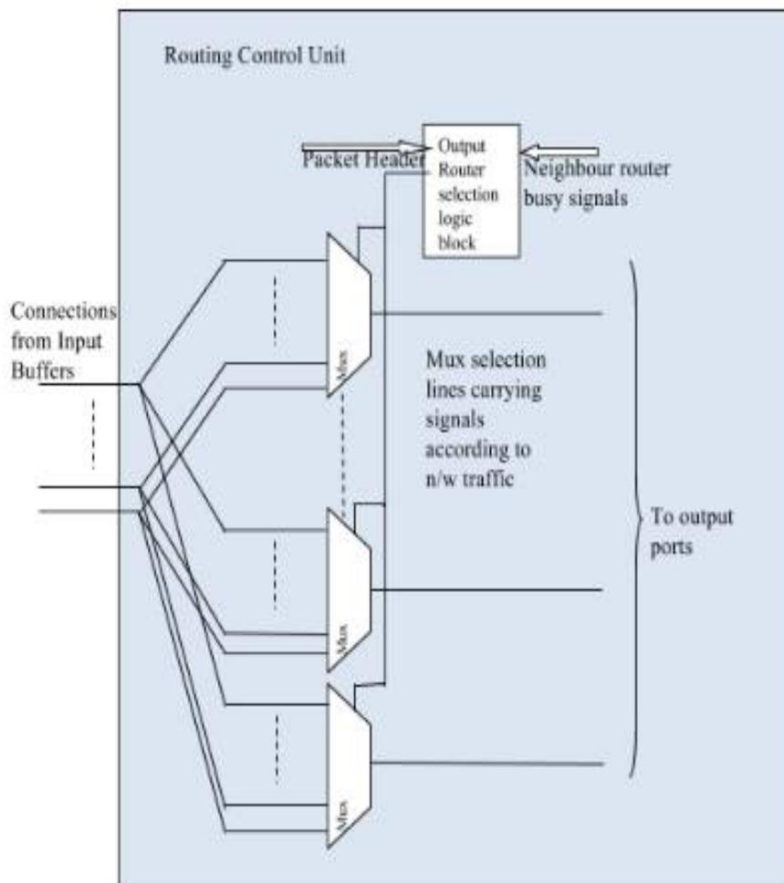
Fig. 8 Router control Unit
