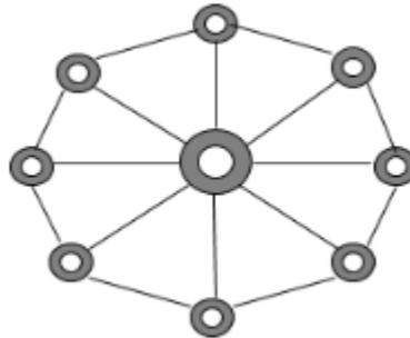
**Figure 3: Spidergon topology with hub at the center for hierarchical network integration, fusion with star topology.**
