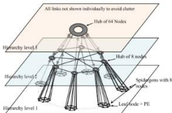
Fig. 9 3D hybrid (hierarchical+spidergon) topology
