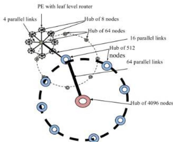
Fig. 6 Spidergon-star hybrid topology with hierarchical & parallel network
