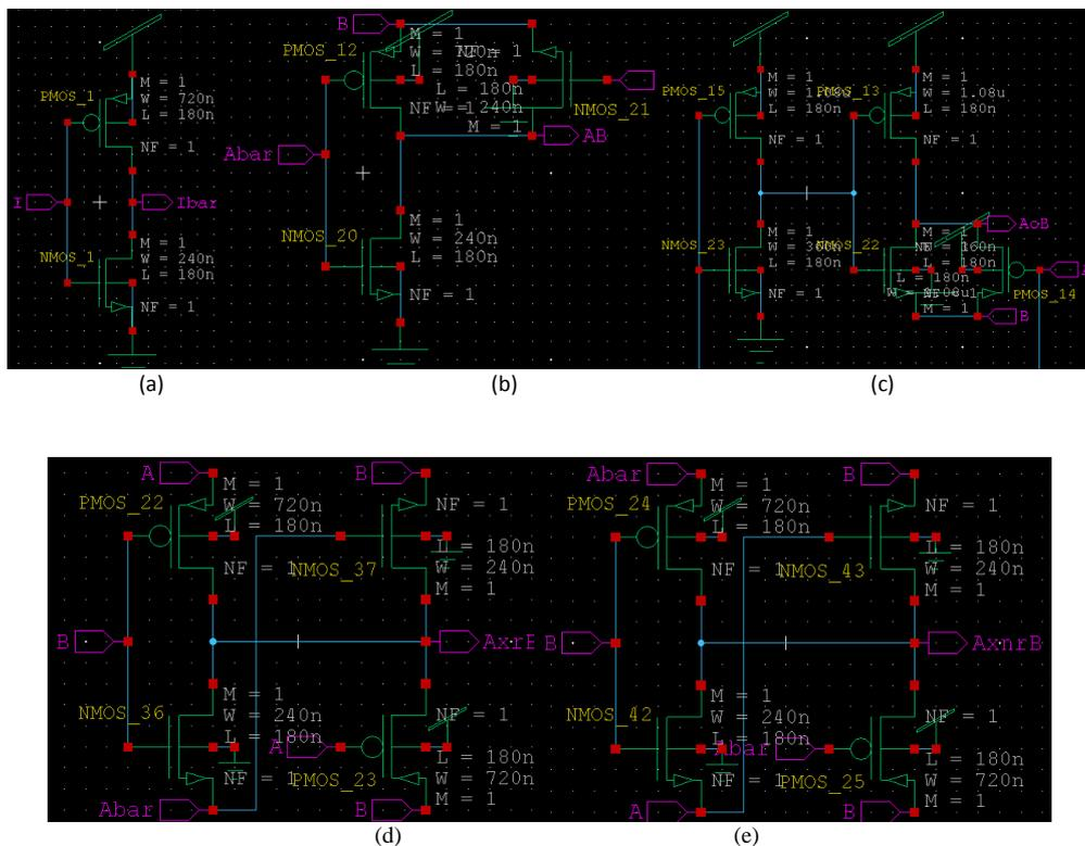
Fig. 5. Implementation of the basic logic gates in Mod-GDI logic
