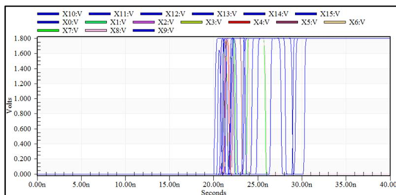
Fig. 8. Simulation results of proposed multiplier for an all 1’s input combination
